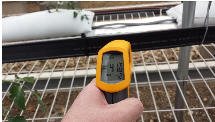
Ambient Heating Ribbon @ 25cm above the perlite Substrate
